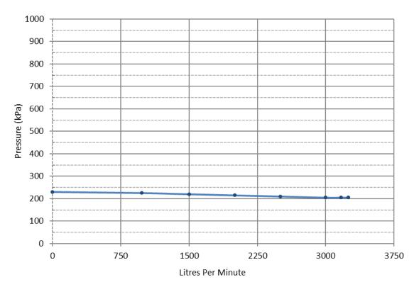
Notes: The hydrants were flowed to full capacity during testing. At full flow H1 was 1750Lpm and H2 was 1500Lpm.
